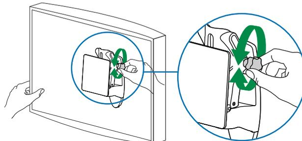
Loosen knob, tilt Display to desired position then retighten knob.
