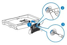
3. After attaching the base, erect the monitor with both hands on holding the monitor together with styrofoam firmly. Now you can pull out the
