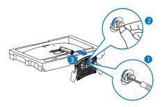
3. Remove the hinge cover from monitor body by using your fingers.
