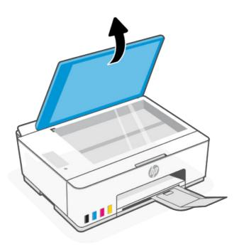
2. Load the original print-side down on the scanner glass (aligned to the indicated corner).
