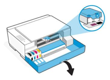
3. Press and release the blue latch to open the printhead cover.
