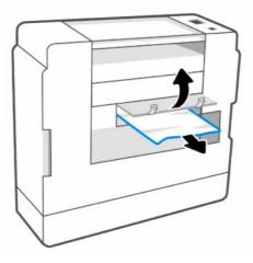
9. Close the bottom access door, making sure the two tabs click into place.
