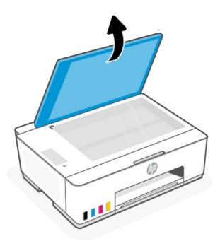
Clean the scanner glass and lid backing by using a dry and soft, lint-free cloth.
