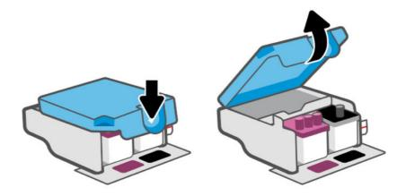
**b.** Remove the printhead from the carriage.
