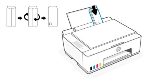
4. Slide the paper-width guide to the right against the stack of envelopes until it stops.
