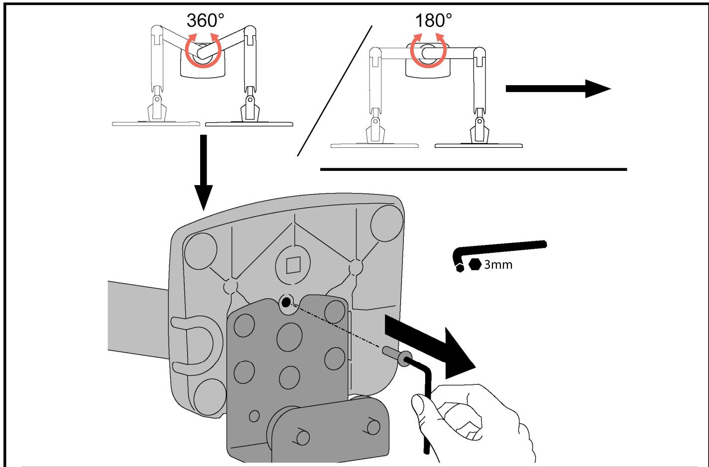
How to replace rotation stop screws (Arms must be straight up)
